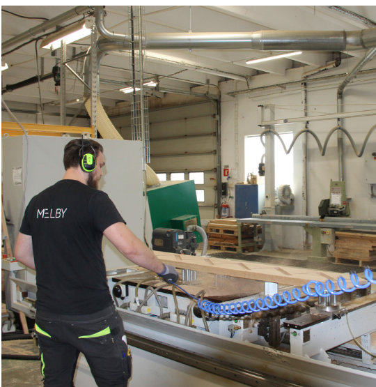
The machine operator can perform other tasks while parts are being processed on the nesting machine. This means that 2 machines can be operated simultaneously by just one person.
