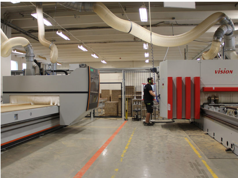
The machine operator can perform other tasks while parts are being processed on the nesting machine. This means that 2 machines can be operated simultaneously by just one person.
